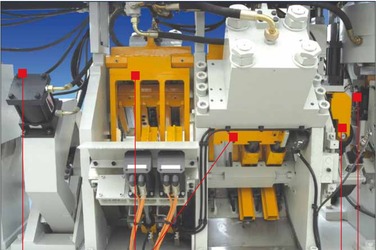
CNC-controlled 38-character marking unit
