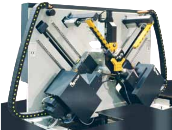
Drilling unit with automatic tool change
