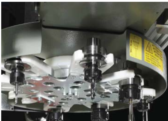
4 or 8 slot round tool holder offers quick tool changes
