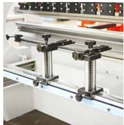
Backgauge Fingers (S) Specifically designed folding backgauge fingers.
