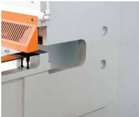
Throat. (standard) 350mm standard throat depth allows you to cut sheet metals that are longer than machine length.
