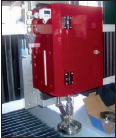
Touch Probe Sensor with Anticollision, Laser Pointer, and Vacuum Assist Tastatore con Anticollusione, Laser e Vacuostato
