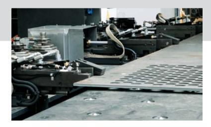
TIPO C16 line is designed to comply with the different requirements when automatically processing in one cycle on large plates ( $3100 \times 1600 \text{ mm.}$ ) and different thicknesses (from 1,5 mm. upto 16 mm.), ensuring high quality, precision, productivity and flexibility.
