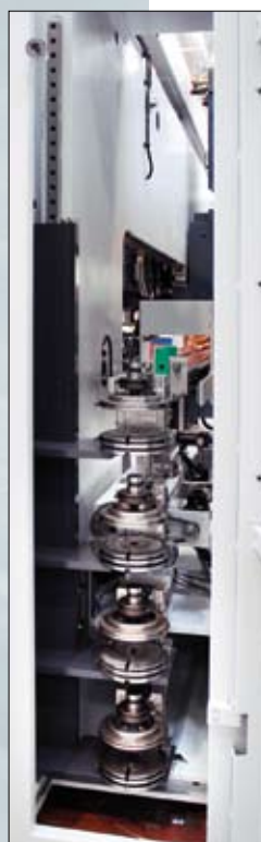
PUNCHING TOOL RACK The tool rack can provide up to 14 different tools, automatically indexes by program command to provide the required tool to the shuttle. Each of the different tool stations can accept punches up to 100 mm in diameter.
