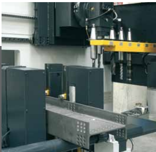
Detail of the drill head during the tool change
