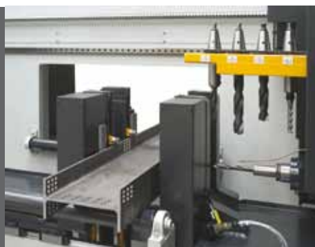
Detail of the drill head during drilling operations on flanges
