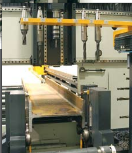
Detail of the drilling head with tool changer
