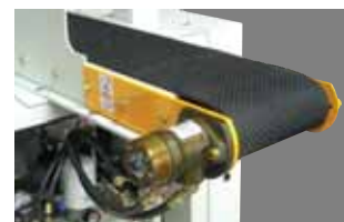
Conveyor Drive Hydraulic Motor
