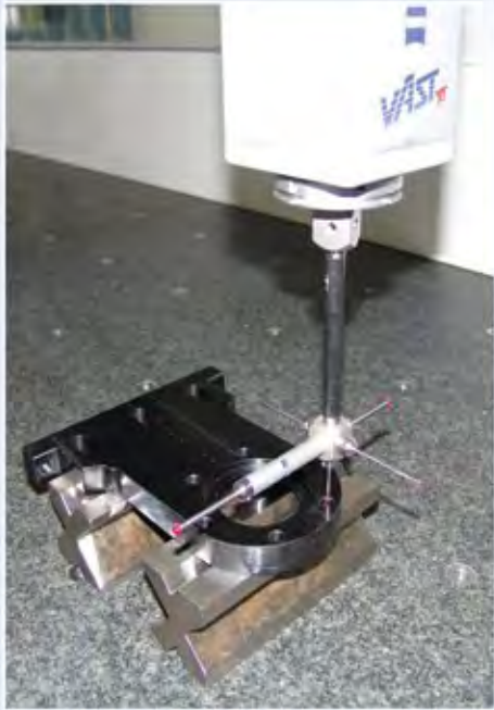
High precision measurement up to 1 micron is feasible with three dimensional measurement device
