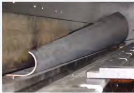
Conical Pole manufacturing with special bottom and top tooling
