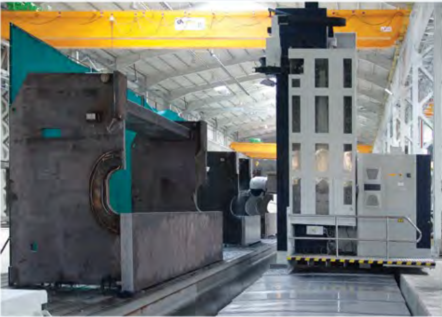
High precision manufacturing up to 28 meter on a single operation at CNC processing centers is feasible.
